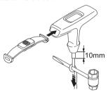
Assemble the starter and tighten the screws.
