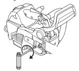
Use the combination spanner to tighten the bar nut while holding up the tip of the bar. Check that you can pull the saw chain round freely by hand, and that there is no slack on the underside of the bar.
