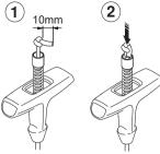
Pull the starter cord against the starter handle so at least 10mm of the spring guide is visible. Insert the starter handle cover.
