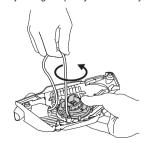
Undo the bolt in the centre of the pulley and remove the pulley.
