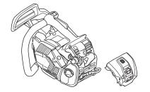
The filter can be cleaned more thoroughly by washing it in water and detergent.
