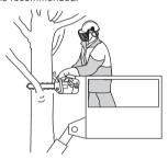
7 Take great care when you cut with the top edge of the bar, i.e. when cutting from the underside of the object. This is known as cutting on the push stroke. The chain tries to push the chain saw back towards the user. If the saw chain is jamming, the saw may be pushed back at you.
